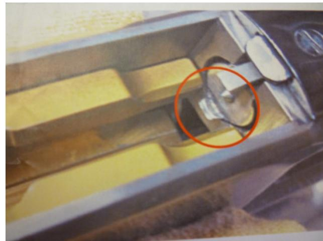
Cycle the lever and check the clearance between the bolt and carrier. Correct timing is achieved when the carrier just misses the bolt as shown in the pictures above. If the carrier hits the bottom of the bolt, you need to remove a small amount of material from the pad of the lifting arm (see picture below). A file, sander or grinder may be used to SLOWLY take away the SMALL amount of material to adjust the timing.
