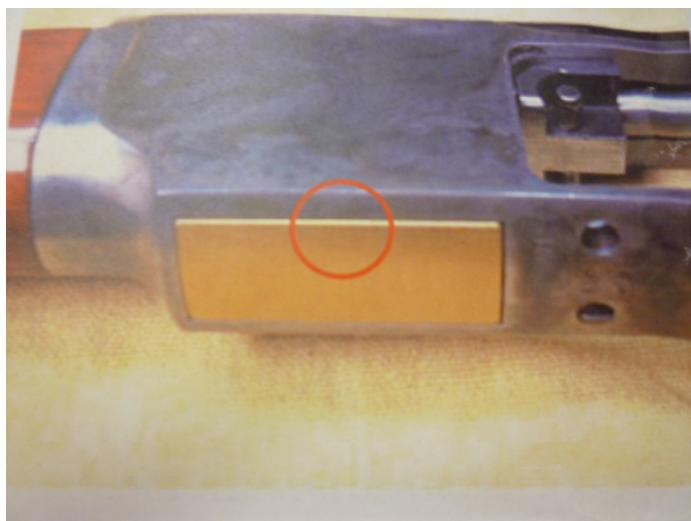
Manually push down on the lifting arm until it bottoms out on the receiver. Check to see that the carrier is approximately flush with the bottom of the receiver (see picture above). If your rifle is a large pistol caliber, it is better if the carrier (both brass and aluminum) is a little below the receiver.
