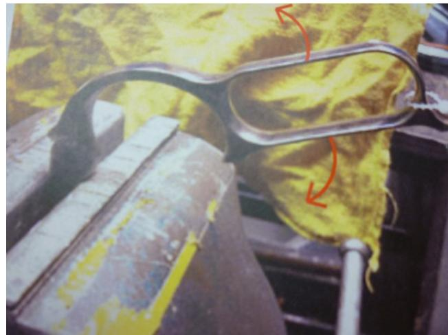
It is important to match the lever to the receiver. The goal is to have about .002-.005" of play between the lever and lifting arm when the lever is closed (see picture above left) or touching the lower tang (see picture below).
